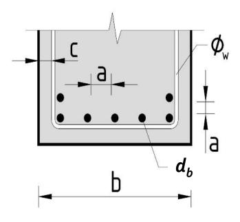
In spirally reinforced or tied reinforced compression members, clear distance between longitudinal bars shall be not less than 1.5d<sub>b</sub>, 4/3d<sub>agg</sub> nor less than 40 mm.
