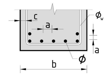
The amount of cover will depend upon the quality of the concrete and the degree of exposure to the elements in the case of rusting. For fire resistance it will depend upon the length of time that the structure is required to resist a fire, the type of concrete aggregate and whether any additional protective covering is to be provided. The following table show the minimum required cover according to ACI 318
